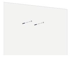
Screw the screws into the anchors using a Phillips screwdriver. Leave the screws sticking out about 1/4"
