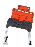
Slide the Vertical Organizer down into position, making sure the tabs securely engage.
