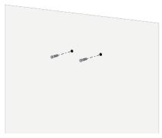
Drill through the marks with a 1/4" drill bit. Then, insert the drywall anchors into the holes and tap them flush with a mallet.
