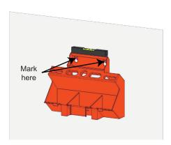
Using a level, hold the Vertical Organizer in the desired location on the wall, then mark inside the mounting holes with a marker or pencil, and remove the Vertical Organizer from the wall.
